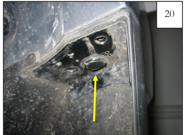
Remove one plastic fastener from mud guard.
