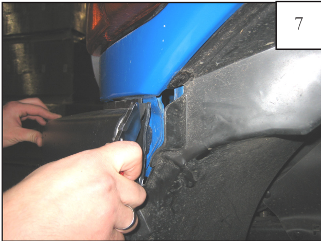
Trim remaining plastic flush with bumper.
