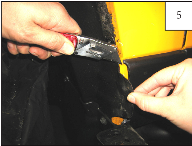
Using a utility knife, cut splash guard flush with edge of sheet metal.
